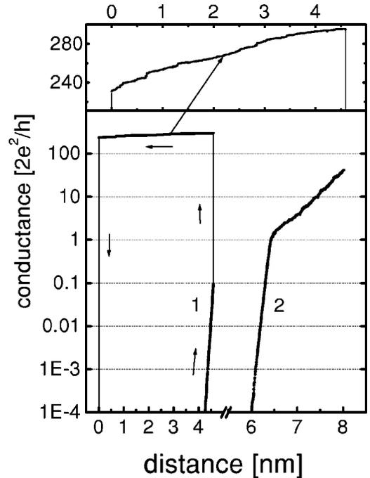
FIG. 2. Two extreme cases of  $G(z)$  traces for W MCBJ. 1: Avalanchelike transition from tunneling to a low-Ohmic contact. The upper panel shows the contact conductance in the process of retraction. 2: Transition from tunneling to direct contact without spontaneous formation of an adhesive neck.
