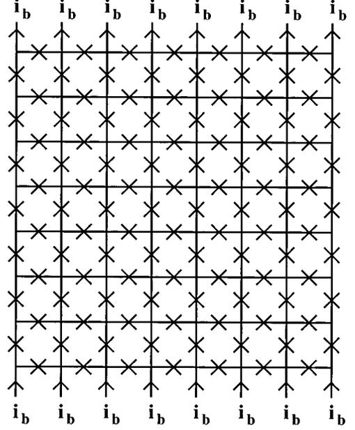
FIG. 1. Square array geometry used in the simulations, illustrated with a  $8 \times 8$  array. Junctions are denoted as crossed bonds. Free boundary conditions are imposed in both directions, while the current bias is applied along the  $y$  direction.
