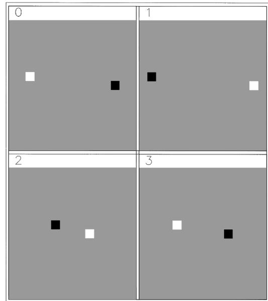
FIG. 6. Snapshots of the vorticity distribution for a  $16 \times 16$  array with free boundaries and  $i_b = 0.65$ , with one positive vortex and one antivortex moving in adjacent rows. The notation is as in Fig. 4. Both vortices reflect at the edges (between frames 0 and 1), and collide constructively in the middle of the array (between 2 and 3), interchanging rows.
