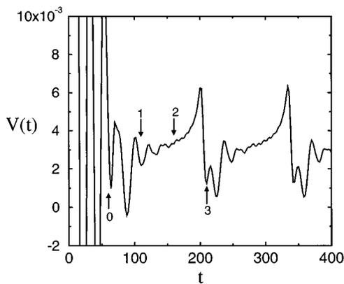
FIG. 5. Voltage, normalized as in Fig. 3, versus time across a  $16 \times 16$  square array with one vortex, for  $\beta_c = 10$  and  $i = 0.49$ . The times labeled with 0 to 3 correspond to the respective snapshots shown in Fig. 4.
