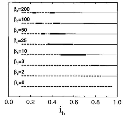
FIG. 2. Results for different values of  $\beta_c$  for a  $16 \times 16$  square array with free boundaries. The dashed lines represent the current ranges for which type-A behavior (vortex escapes from array) was found. The thick lines denote the type-B ranges (trapped vortex oscillating in the array) and the thin solid lines the row-switching regimes.
