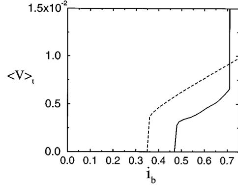
FIG. 3. Current-voltage characteristics for  $\beta_c = 10$ , from simulations of a  $16 \times 16$  square array with one vortex (solid line).  $\langle V \rangle_t$  is the time-averaged voltage across the array in the current direction, in units of  $I_c R_n$  and normalized by the number of longitudinal junctions. The dashed line is the  $I$ - $V$  characteristic computed from the linear viscosity model (11).
