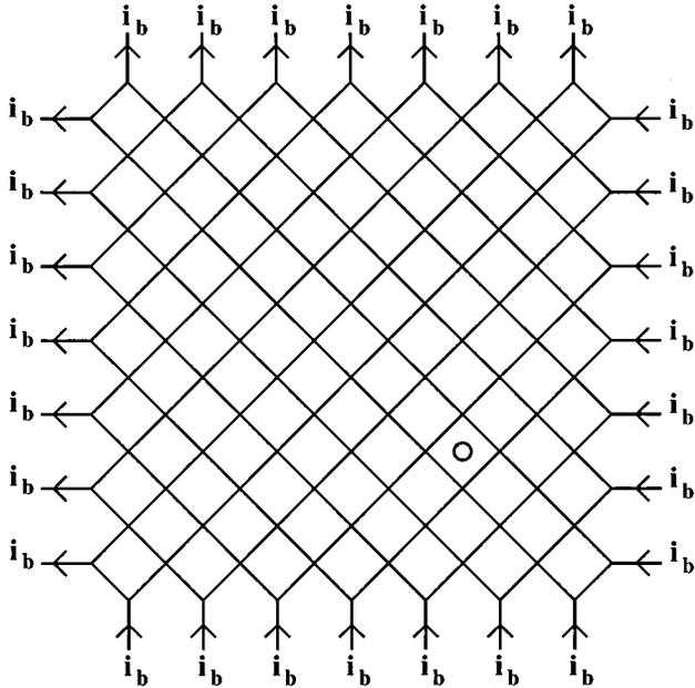
FIG. 9. Diagonal array geometry used in the simulations, illustrated with a  $15 \times 15$  array. For clarity we omitted the crosses on the bonds. In both directions free boundary conditions are imposed, while the current bias is applied along a diagonal direction. The open circle denotes the initial position of the vortex.
