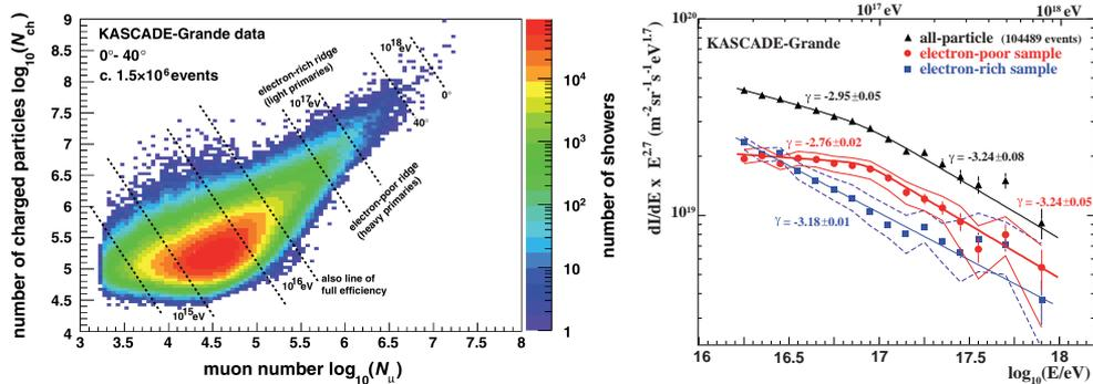
**Fig. 3.** Left: The two-dimensional shower size spectrum for KASCADE-Grande data. Right: The energy spectra for all particles, light (electron-rich) and heavy (electron-poor) primaries based on the two-dimensional spectrum on the left side (See [10]).
