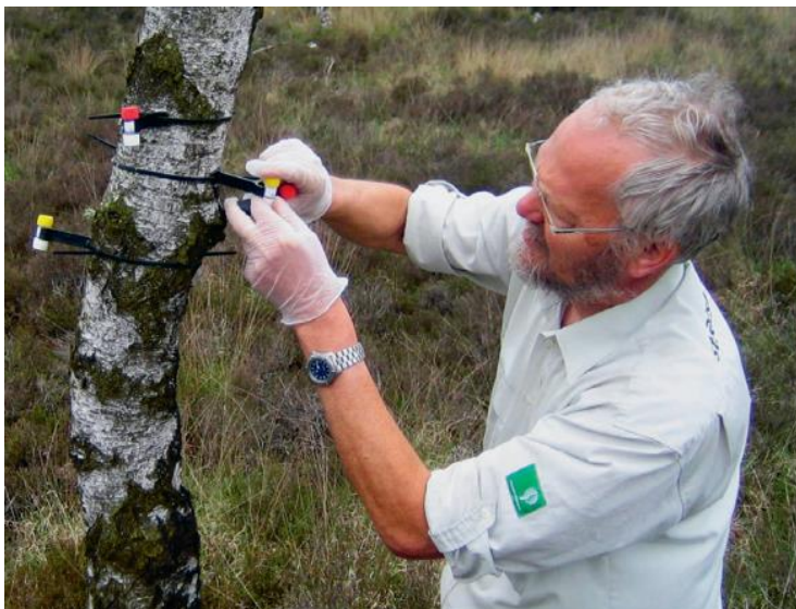
Figure 1: A ranger exchanging a passive ammonia sampler
