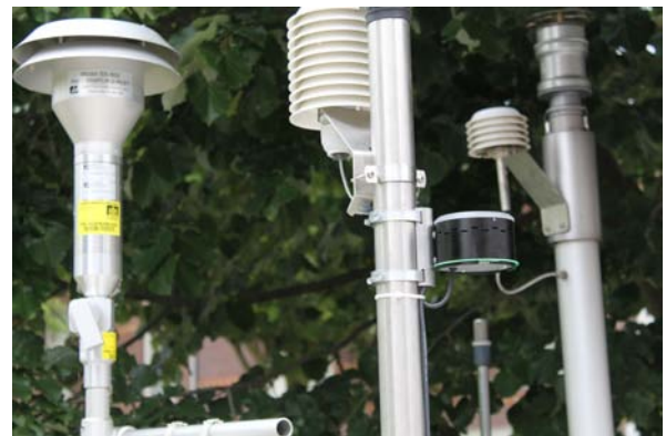
Fig. 1. Smart Emission Jose sensor (top) and Jose sensor installation at site of the national air quality network (bottom)
