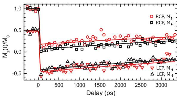
FIG. 3. Polarization dependence of the magnetization dynamics after a single 60 fs laser pulse excitation. The RCP and LCP optical pump pulses are used to excite the multilayer, which magnetization is saturated parallel  $\vec{M}_\uparrow$  or antiparallel  $\vec{M}_\downarrow$  to the sample normal. The magnetization dynamics for LCP laser excitation is shifted down by 0.5 for a better visual representation.
