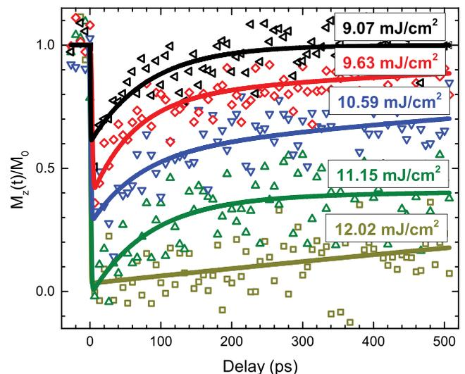
FIG. 2. The laser fluence dependence of the magnetization dynamics reconstructed from magneto-optical images (see calibration procedure explanation in the text). The ultrafast demagnetization scales with the laser fluence.
