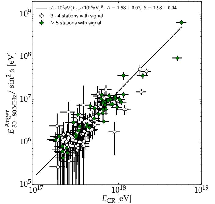
FIG. 2. Correlation between the normalized radiation energy and the cosmic-ray energy  $E_{\text{CR}}$  as determined by the Auger surface detector. Open circles represent air showers with radio signals detected in three or four radio detectors. Filled circles denote showers with five or more detected radio signals.
