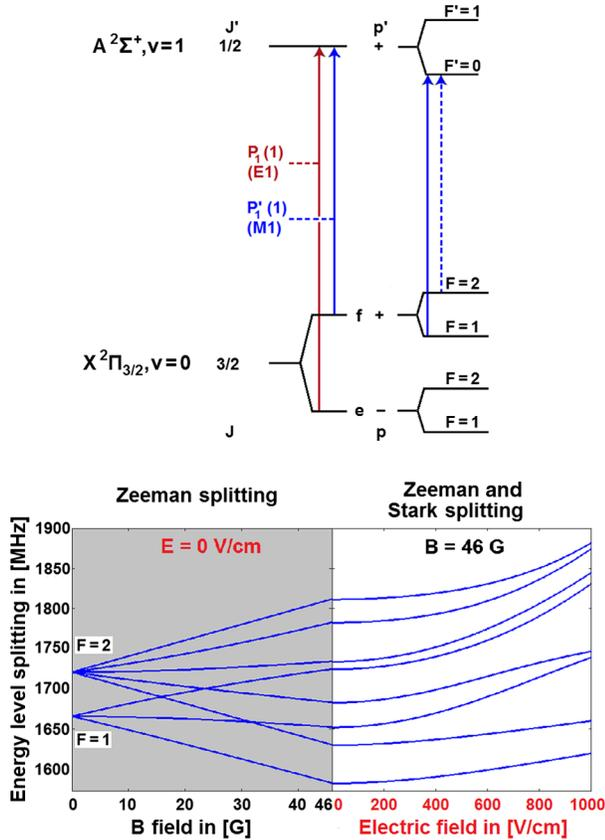
FIG. 1. The upper drawing shows the ground ( $X^2\Pi_{3/2}, v=0$ ) and excited ( $A^2\Sigma^+, v'=1$ ) states and the electric and magnetic dipole transitions investigated. The bottom picture shows the eight split energy levels (blue curves) of the upper  $\Lambda$ -doublet component of the ground state in perpendicular static electric and magnetic fields.
