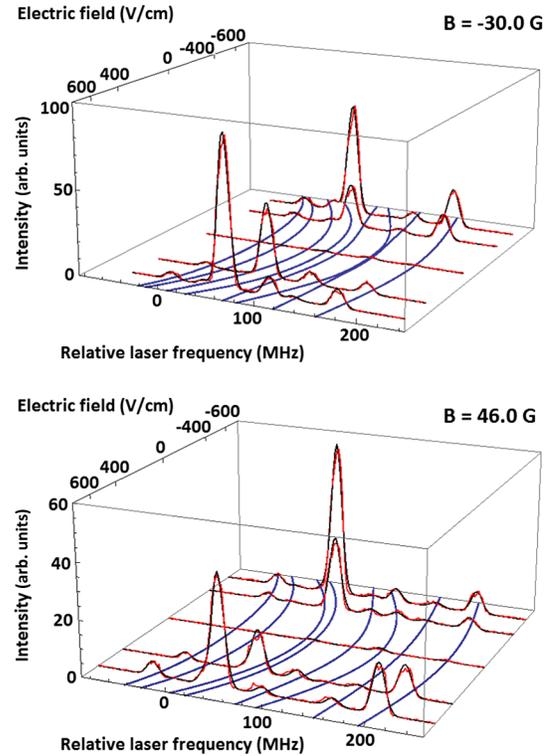
FIG. 3. Measured (red lines) and fitted (black lines) spectra as function of the static electric field strength  $E_{\text{stat}}$ , for two different static magnetic field values. The blue curves under each of the eight peaks indicate the calculated center frequencies of the transitions originating from each of the eight hyperfine levels in the ground state (shown in Fig. 1) to the single, nondegenerate  $F' = 0$  hyperfine level in the excited state. The intensity is given in arbitrary units.
