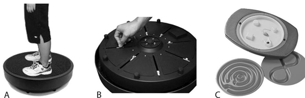
Fig. 1. A) Pro-balance. The tilt of the platform was represented by a cursor on the screen. The cursor was moved using center of gravity displacements. Games were either aimed at making smooth and precise movements or quick weight shifts. B) Sliders on the bottom of the system enabled us to change the stability of the platform and adjust it to the participants' performance level. C) Balanco balance board with 3 interchangeable game surfaces through which a ball can be directed by making weight shifts.
