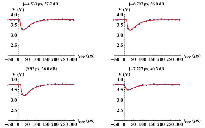
FIG. 4. (Color online) Four fits of the voltage drop chosen at random. The red line is the best fit voltage, the blue points are the measured values. Each graph is labeled by  $\{t_d, A_2\}$ , where  $t_d$  is the interpulse delay in picoseconds and  $A_2$  is the total attenuation. An example of the corresponding conduction band density is shown in Fig. 5.
