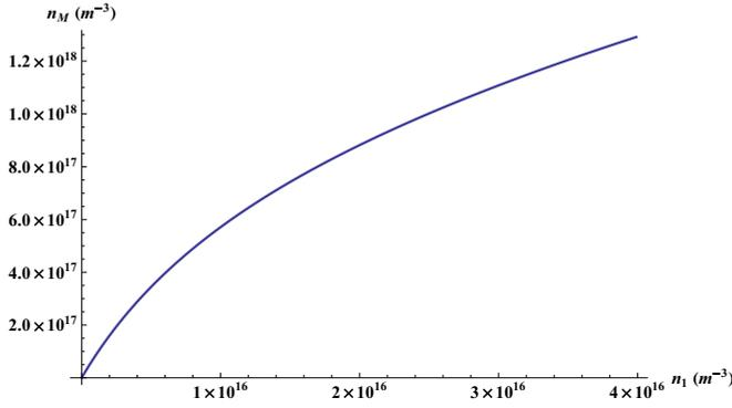
FIG. 3. (Color online) The effective multipulse ionization density  $n_M$  as a function of initial single pulse ionization density  $n_1$ , for  $M = 100$  micropulses separated by 40 ns. We assume  $n_{\text{eq}} = 3 \times 10^{16} \text{ m}^{-3}$ ,  $n_c = 5 \times 10^{16} \text{ m}^{-3}$ , and  $P = 5.3 \times 10^{-13} \text{ m}^3 \text{ s}^{-1}$ , values typical of these experiments.
