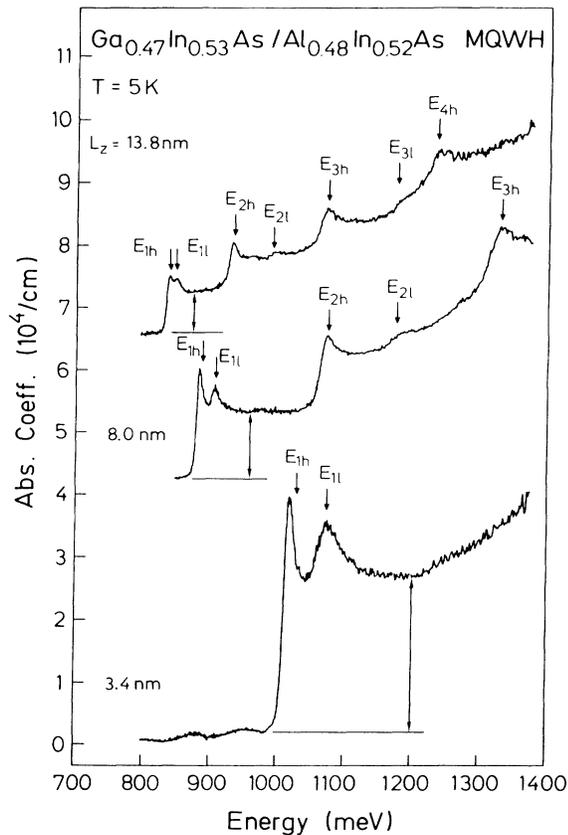
FIG. 1. Absorption spectra of three  $\text{Ga}_{0.47}\text{In}_{0.53}\text{As}/\text{Al}_{0.48}\text{In}_{0.52}\text{As}$  MQWH's with different well widths  $L_z$  at 5 K. The arrows indicate experimentally determined subband transitions.
