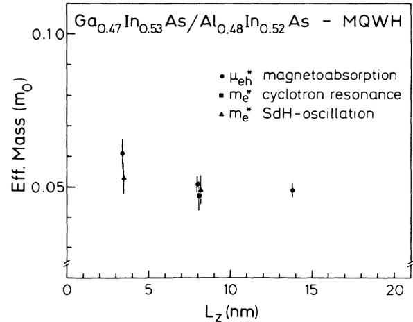
FIG. 6. Carrier effective masses of a  $\text{Ga}_{0.47}\text{In}_{0.53}\text{As}/\text{Al}_{0.48}\text{In}_{0.52}\text{As}$  MQWH as a function of the well width.
