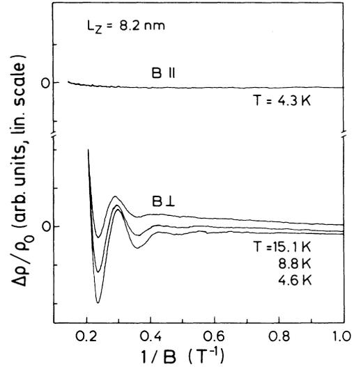
FIG. 5. Magnetoconductance measurements of a modulation-doped  $\text{Ga}_{0.47}\text{In}_{0.53}\text{As}/\text{Al}_{0.48}\text{In}_{0.52}\text{As}$  MQWH ( $L_z = 8.2$  nm) for two different orientations of the magnetic field with respect to the well layers at various temperatures.
