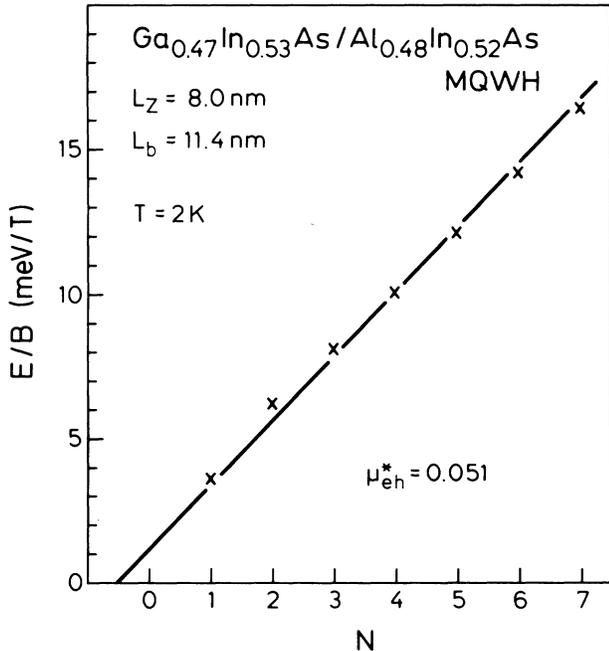
FIG. 4. Slope of the Landau level fan as a function of the Landau quantum number  $N$  for a  $\text{Ga}_{0.47}\text{In}_{0.53}\text{As}/\text{Al}_{0.48}\text{In}_{0.52}\text{As}$  MQWH with  $L_z = 8$  nm.
