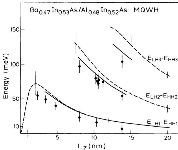
FIG. 3. Energy difference between light- and heavy-hole valence subbands of the same quantum number for a  $\text{Ga}_{0.47}\text{In}_{0.53}\text{As}/\text{Al}_{0.48}\text{In}_{0.52}\text{As}$  MQWH as a function of the well width (dashed line, parabolic single-band envelope-function approximation; solid line, coupled six-band envelope function approximation).
