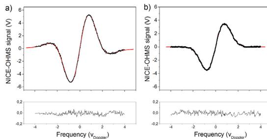
Fig. 2. NICE-OHMS signal of 200 ppbv methane at  $6123.3 \text{ cm}^{-1}$  for dispersion (panel a) and absorption (panel b) as a function of Doppler frequency (473 MHz). Black dots represent measurement points, with a fit in red. Residuals of each plot are given below.
