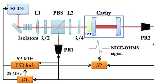
Fig. 1. Schematic of the NICE-OHMS setup employing solely current modulation. ECDL: External Cavity Diode Laser; PBS: Polarizing beam splitter; PZT: Ring piezoelectric transducer;  $\lambda/2$  and  $\lambda/4$ : Half wave and quarter wave plate; PR1 and PR2: Photoreceivers 1 and 2; DL: Toptica Digilock; SP: Signal processor, L1 and L2: mode-matching lenses.
