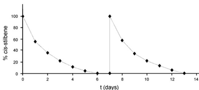
**Figure 5.** Epoxidation of twice 250 equivalents of *cis*-stilbene by **MnDC** in the presence of one equivalent of **py**. Epoxidation of a second batch reveals an identical rate (within 15%) of epoxidation, highlighting the stability of the catalyst.
