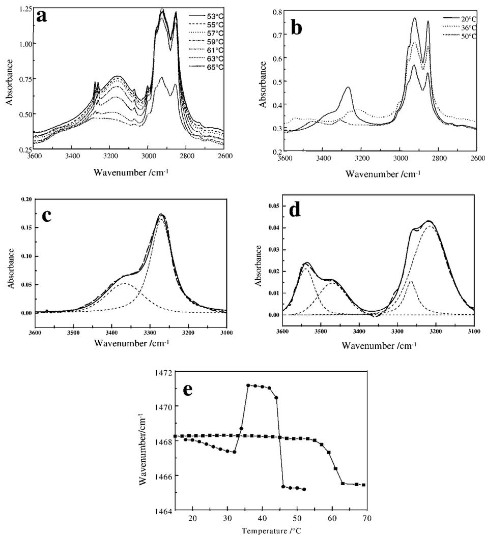
**Fig. 3** Variable temperature FT-IR spectra of annealed films of (a) **1b** and (b) **1c**. Overlay of experimental and fitted FT-IR spectra of **1c** at (c) 20 °C and (d) 36 °C. (e) Temperature dependence of the position of the CH<sub>2</sub> deformation band in the FT-IR spectra of (■) **1b** and (●) **1c**.
