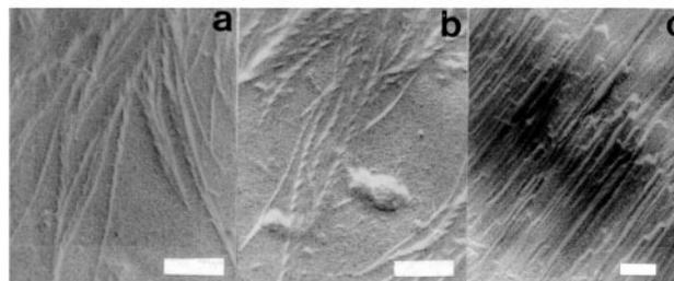
**Fig. 7** Electron micrographs taken from 0.1% dispersions of **1b** and **2** in water (platinum shadowing, bars represent 250 nm). (a) Left-handed and (b) right-handed helices from **1b** and aspirin; (c) rod-like structures from **2**.
