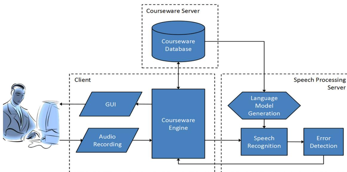
Figure.1. A schematic overview of the GREET system
