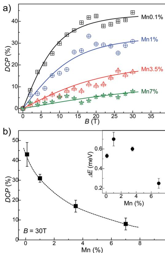
Fig. 5 (a) Degree of circular polarization (DCP) data at  $T = 7$  K averaged over 4 repeats. Curves are fitted by the method of least squares with two free fitting parameters:  $\tau_s/\tau$  and  $g_x$ . (b) Dependence of the DCP on Mn-content and (inset) Zeeman splitting,  $\Delta E$ , at  $B = 30$  T and  $T = 7$  K. Error bars represent a standard deviation of 4 measurements.
