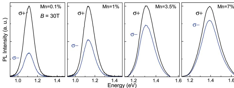
Fig. 4 Polarised ( $\sigma^+$  and  $\sigma^-$ ) PL spectra for PbS:Mn QDs with different Mn-content at  $B = 30$  T and  $T = 7$  K. For clarity, the PL spectra are normalised to the peak intensity of the  $\sigma^+$  PL spectrum.
