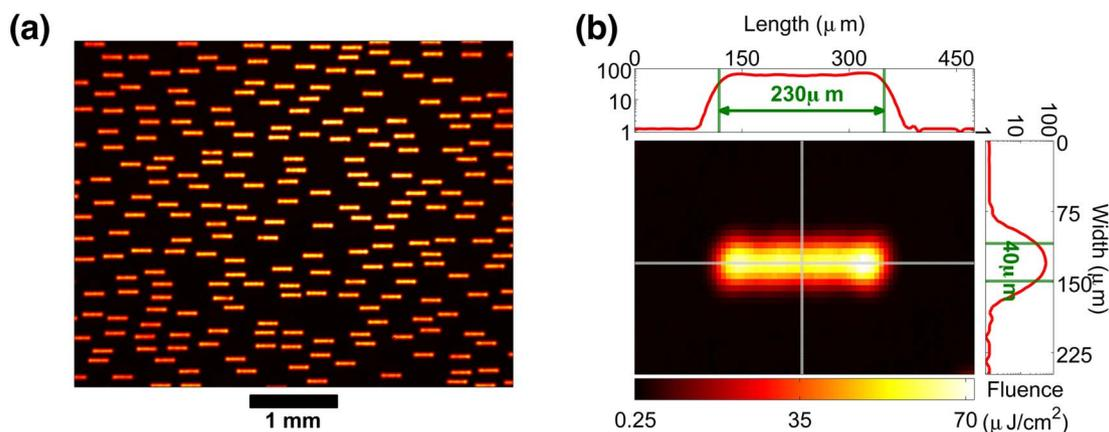
**Figure 2** | (a) Image of a random array of photo-generated rods. (b) Close view image of a single rod. The upper and right plots are the intensity profiles along the horizontal and vertical dotted lines. The vertical axis and the color scale indicate the pump fluence in  $\mu\text{J}/\text{cm}^2$ . The dimensions of the rods are defined by the FWHM of the pump beam intensity marked by the vertical dashed lines.
