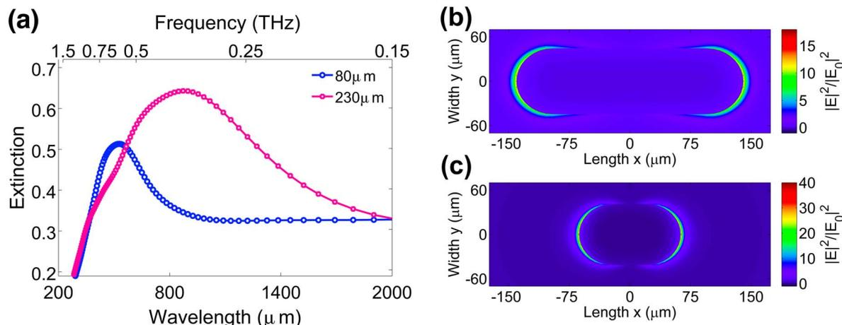
**Figure 5** | Finite difference in time domain simulations of photo-generated rods. (a) Simulated extinction for rods with effective dimensions  $230 \times 40 \mu\text{m}^2$  and  $80 \times 40 \mu\text{m}^2$ . (b) simulated total field enhancement at the GaAs-air interface for a rod with an effective length of  $230 \mu\text{m}$ . (c) same as (b) but for a rod with an effective length of  $80 \mu\text{m}$ .
