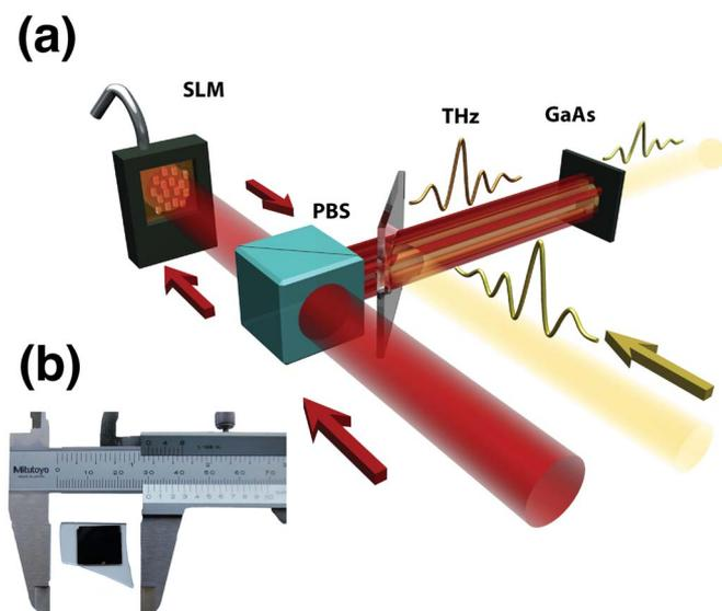
**Figure 1** | (a) Schematic representation of the setup used for photo-generation of THz linear antennas. The optical pump is indicated by the red beam, whose profile is structured by the spatial light modulator (SLM). Collinear to the optical pump is a THz pulse represented by the yellow beam. (b) Photograph of the GaAs layer used as sample to photo-generate plasmonic antennas.
