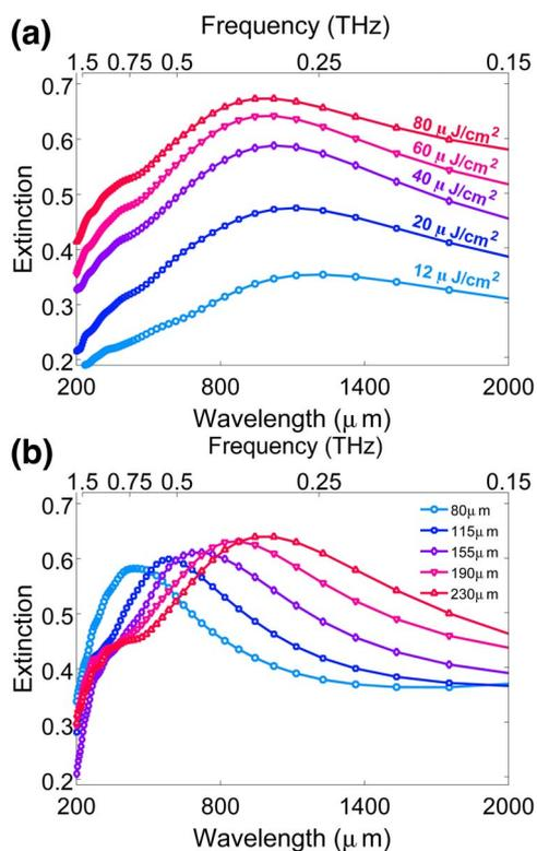
**Figure 3** | Extinction spectra of photo-generated rods on a layer of undoped GaAs. (a) The dimension of the rods is kept fixed to  $230 \times 40 \mu\text{m}^2$  and the pump fluence is varied. (b) The pump fluence for the photo-generation of the rods is  $70 \mu\text{J}/\text{cm}^2$  for all the samples and the length of the rods is varied.
