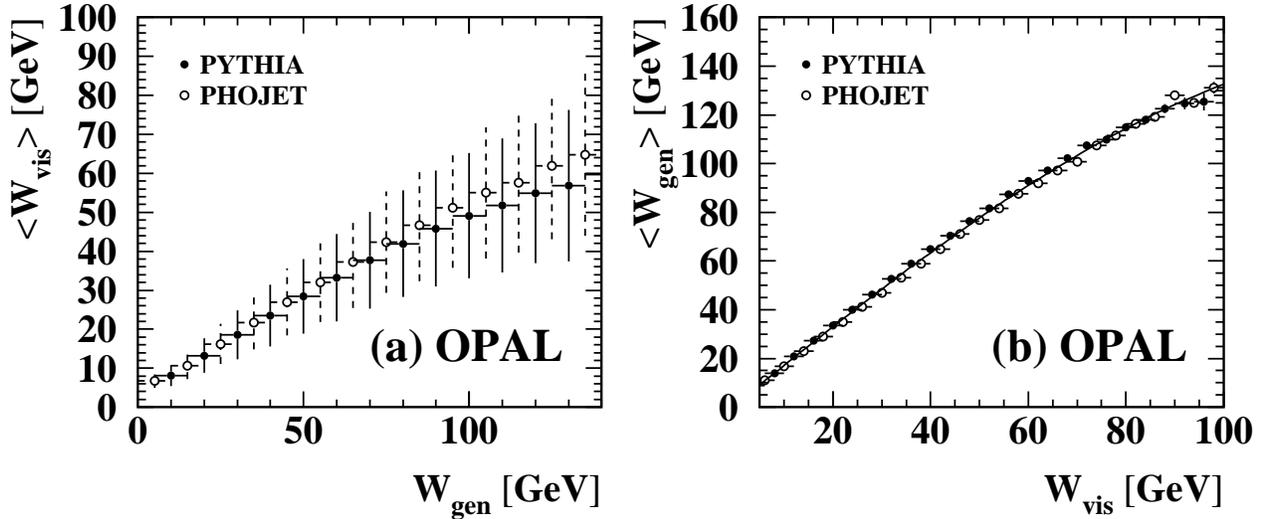
Figure 1: The relation between the generated hadronic invariant mass  $W_{\text{gen}}$  and the visible hadronic invariant mass  $W_{\text{vis}}$  for PHOJET and PYTHIA Monte Carlo events. The vertical bars show the standard deviation in each bin in (a) and the error on the mean in (b). The polynomial fit shown in (b) determines the correction function for  $W_{\text{vis}}$ .
