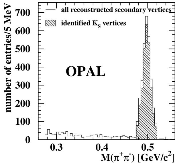
Figure 2: Distribution of the  $\pi^+\pi^-$  invariant mass  $M$  for all identified secondary vertices in the selected events before (open histogram) and after (hatched histogram) applying the cut  $|M(\pi^+\pi^-) - 0.4977 \text{ GeV}/c^2| < 0.02 \text{ GeV}/c^2$  and the  $dE/dx$  cuts used to identify  $K_S^0 \rightarrow \pi^+\pi^-$  vertices.
