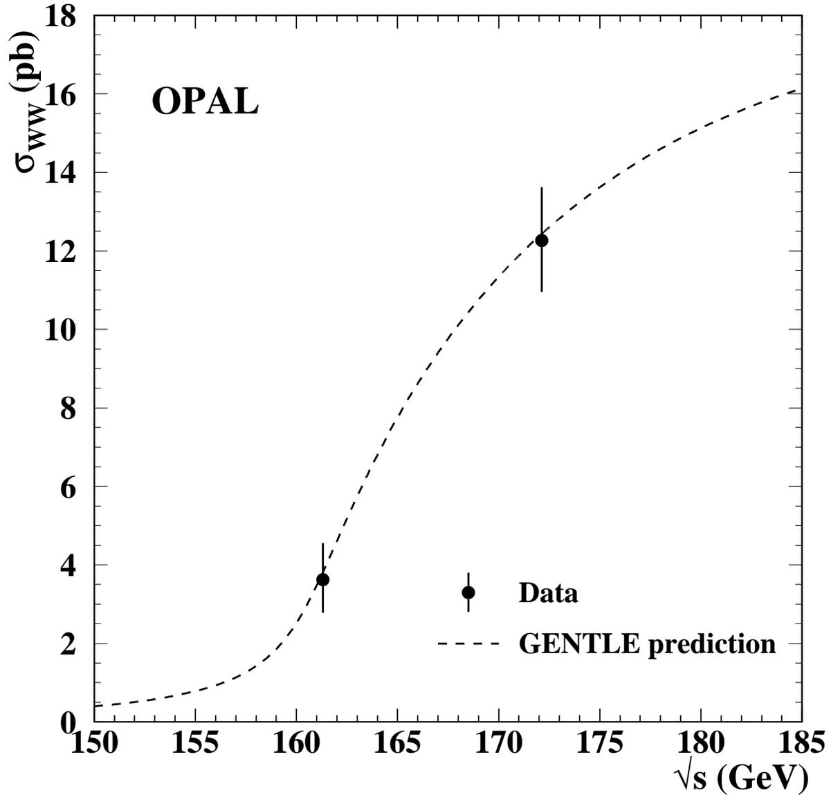
Figure 4: The dependence of  $\sigma_{WW}$  on  $\sqrt{s}$ , as predicted by GENTLE for  $M_W = 80.33$  GeV. The  $W^+W^-$  cross-sections measured at  $\sqrt{s} = 172.12$  GeV (this paper) and at  $\sqrt{s} = 161.3$  GeV [5], are shown. The error bars include statistical and systematic contributions.
