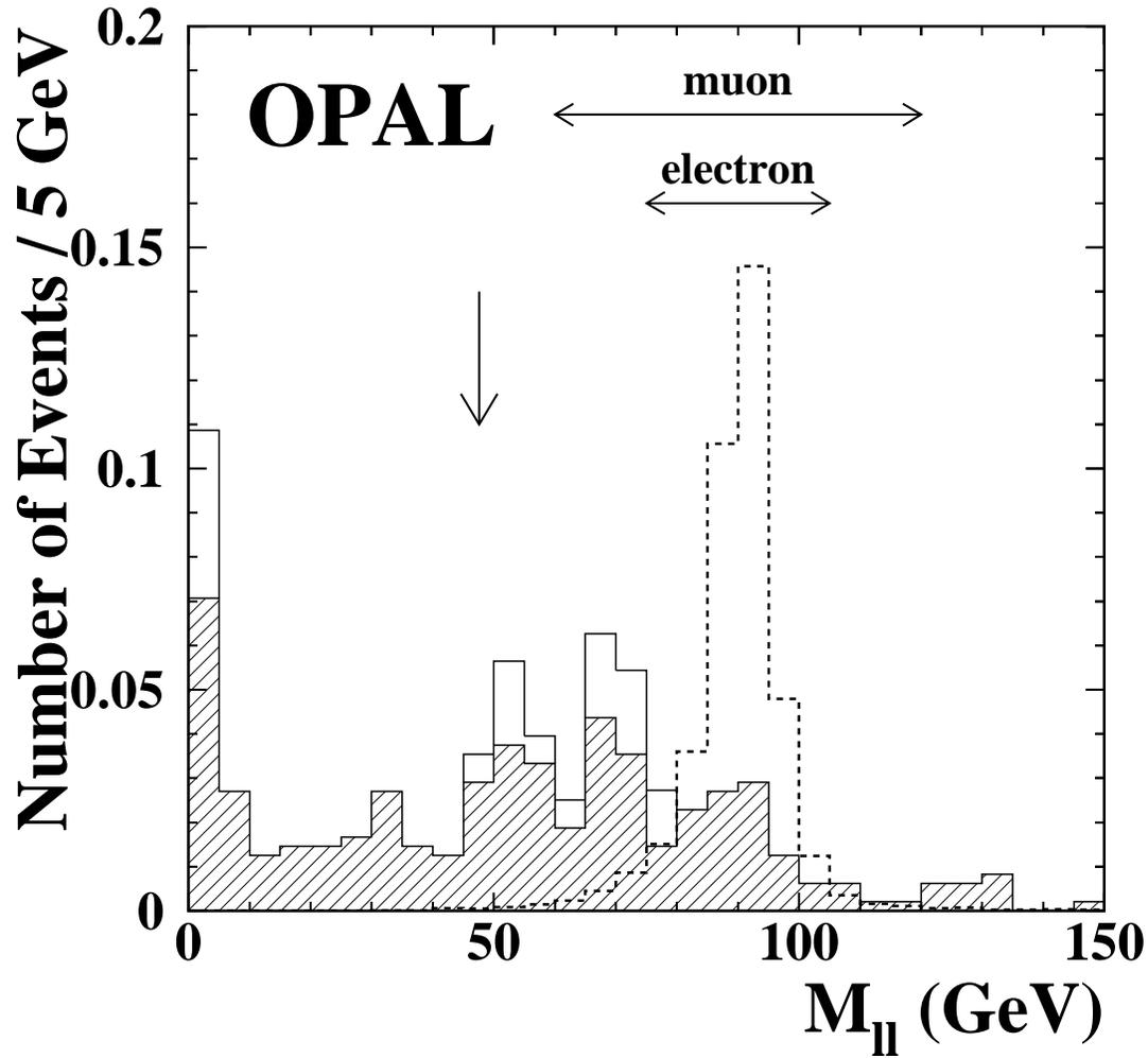
Figure 10: Electron and muon channels; invariant mass of the lepton pair, after cut (4). Open / shaded / dotted histograms:  $Z^0/\gamma^* \rightarrow q\bar{q}$  / four-fermion backgrounds / simulated signal ( $m_{H^0}=68$  GeV,  $e^+e^-$  and  $\mu^+\mu^-$  channels combined). All simulations are normalized to the integrated luminosity. Horizontal arrows: selected mass ranges; vertical arrow: invariant mass of the event remaining in the  $e^+e^-$  channel after cut (4).
