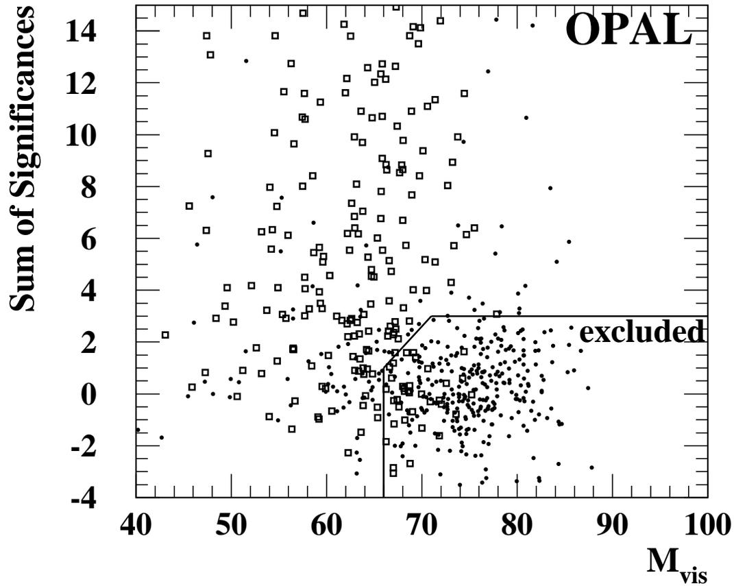
Figure 6: Missing energy channel; scatter plot of  $\Sigma_S$  vs. the visible mass, after cut (7); dots: simulated four-fermion background; open squares: signal for  $m_{H^0}=68$  GeV. straight line: cut region. The one event (not shown) which survived the cuts, is at a visible mass of 67.7 GeV and  $\Sigma_S=1.6$ .
