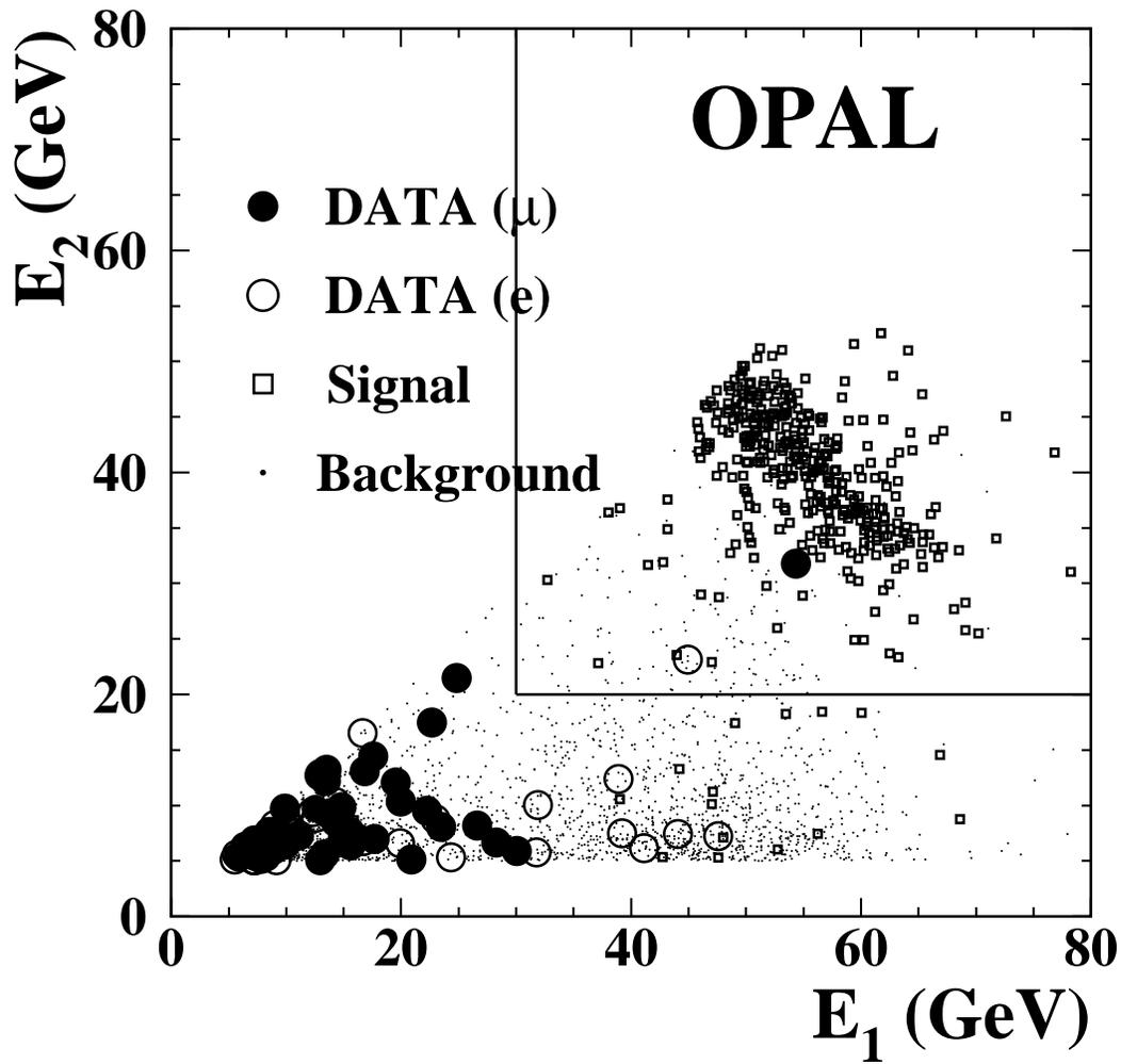
Figure 9: Electron and muon channels; scatter plot of the energies of the lepton candidates, after cut (2). The symbols for the data and the simulated signal ( $m_{H^0}=68$  GeV,  $e^+e^-$  and  $\mu^+\mu^-$  channels combined) as indicated; small dots: simulated backgrounds. Solid lines: position of cut (3).
