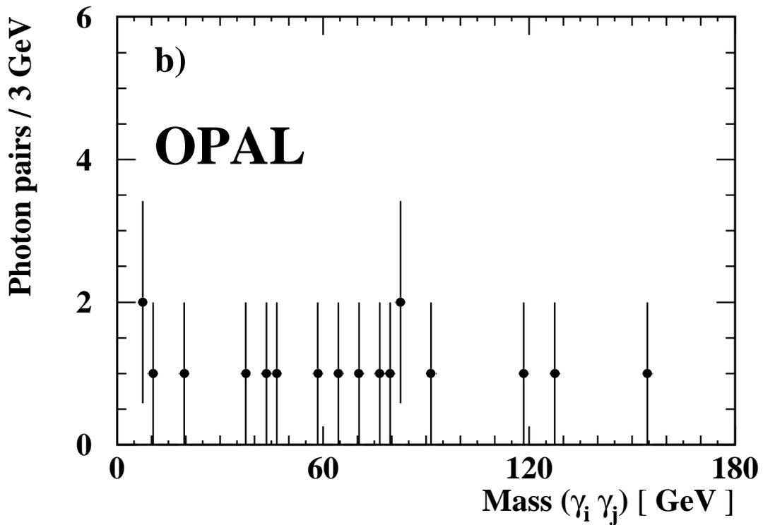
Figure 5: The invariant mass of photon pairs from a) class-III and b) class-IV events. The points are the data and the open histogram the  $e^+e^- \rightarrow \gamma\gamma(\gamma)$  Monte Carlo expectation scaled by a factor of two for clarity. The hatched histogram in a) represents a  $\gamma\gamma$  resonance at 95.5 GeV with a cross-section times branching ratio of 0.10 pb. In each case, the binning is chosen to match the expected mass resolution.
