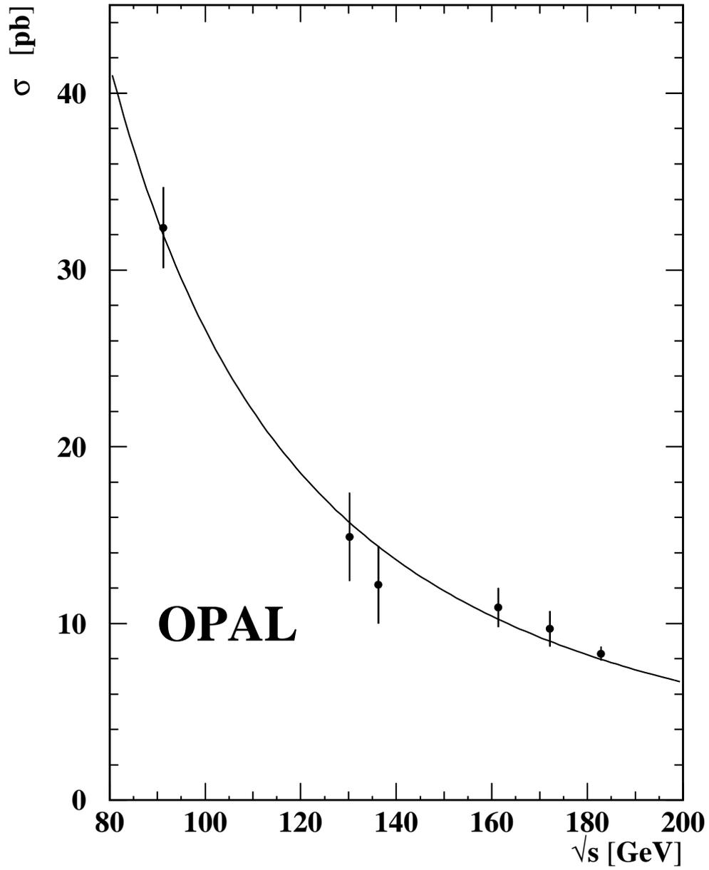
Figure 2: Total cross-section for the process  $e^+e^- \rightarrow \gamma\gamma$  with  $\cos\theta^* < 0.9$ . The data are corrected for efficiency loss and higher-order effects and correspond to Born level. Results at lower energies are taken from [5, 22]. The curve shows the Born-level QED expectation.
