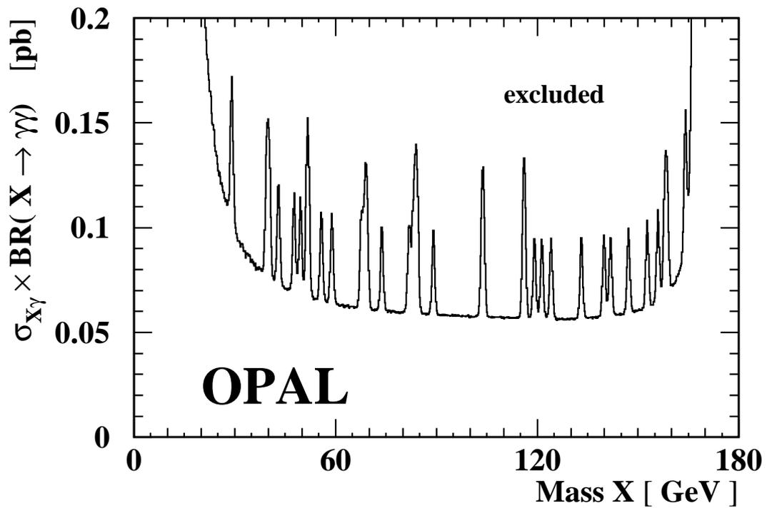
Figure 6: Upper limit (95% CL) for the cross-section times branching ratio for the process  $e^+e^- \rightarrow X\gamma$ ,  $X \rightarrow \gamma\gamma$  as a function of the mass of the resonance X. Only class-III events are used for this result.
