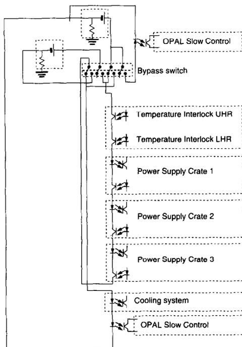
Fig. 6. Schematic of the OPAL microvertex interlock system.
