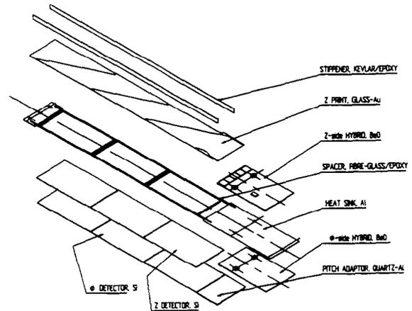
Fig. 2. Exploded view of an OPAL long ladder.
