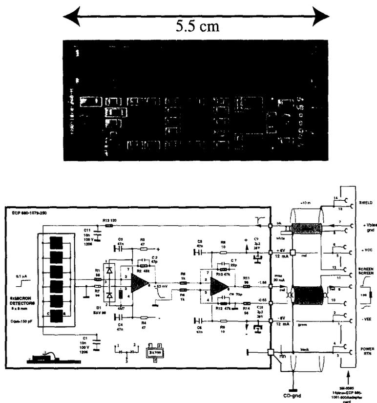
Fig. 7. Radiation monitor front end cards in real life (top picture) and in schematics (bottom picture).
