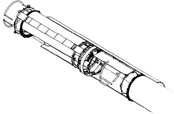
Fig. 4. The OPAL Phase III microvertex detector schematic view. Only one long and short ladder pair is shown and one ICR card.
