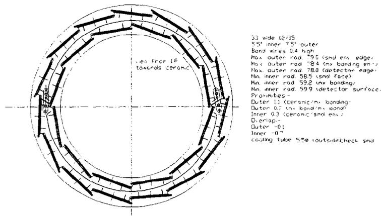
Fig. 1. Cut in the transverse direction of the OPAL silicon microvertex detector. The constraining space is formed by the wall of the pressure vessel on the outside and the beam pipe on the inside.
