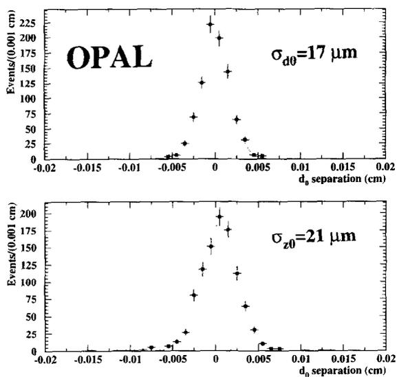
Fig. 8. Impact parameter resolution in the plane transverse to the beam ( $d_0$ ) and in the direction along the beam ( $z_0$ ) for  $e^+e^- \rightarrow Z^0 \rightarrow \mu^+\mu^-$  events, where the  $\mu$  tracks are perpendicular to the beam direction.
