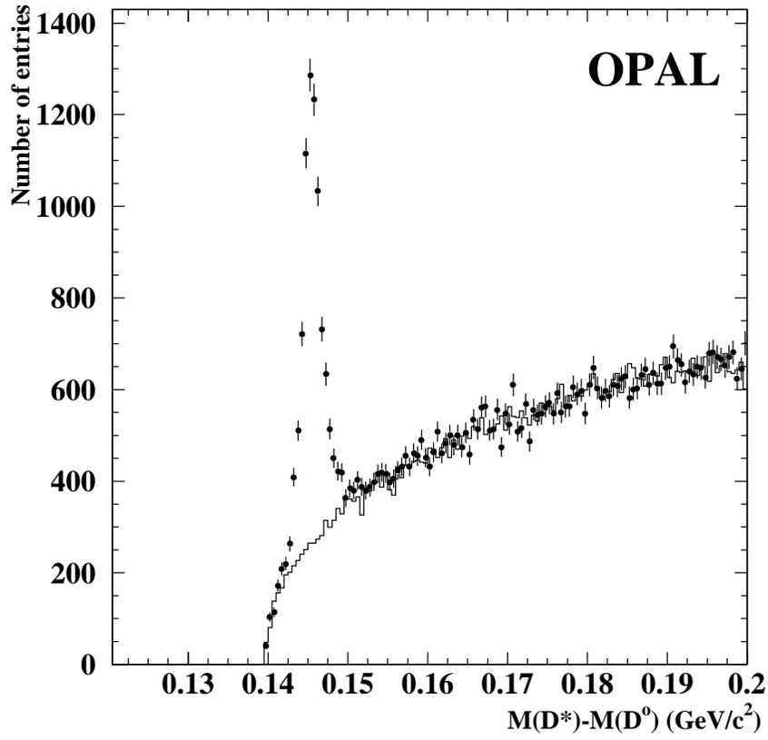
Figure 3: Mass difference distribution for the  $D^*$  candidates with  $x_E > 0.2$ , before applying the  $\Delta M$  cut. The points show the signal sample and the line histogram the distribution of the background obtained from wrong-charge, reflected pion and reflected pion wrong-charge combinations. The errors on the data points are statistical only.
