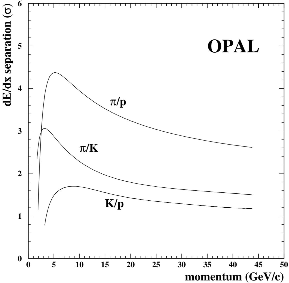
Figure 1: Two particle separation power  $(dE/dx_1 - dE/dx_2)/\langle\sigma(dE/dx)\rangle$  in units of mean  $dE/dx$  resolution as a function of particle momentum for tracks with  $|\cos\theta| < 0.7$  and at least 20 measured samples, obtained from data. The curves given are for pion/proton, pion/kaon and kaon/proton separation.
