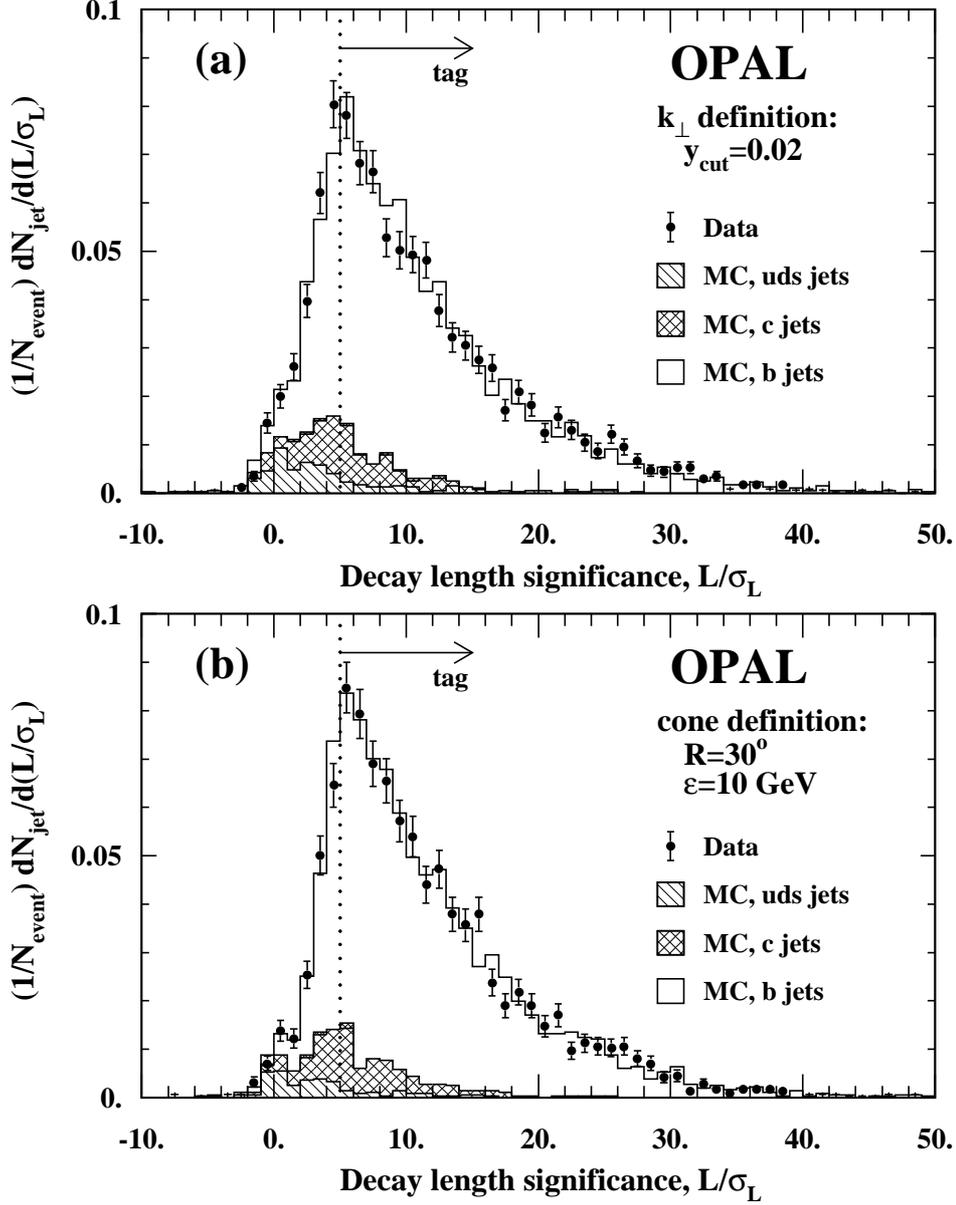
Figure 1: (a) Decay length significance distribution for the highest energy jets of the normal-mixture sample, defined using the  $k_{\perp}$  jet finder, compared to the prediction of the Jetset 7.3 Monte Carlo including detector simulation, after the cuts described in the text have been applied. (b) Corresponding distribution for the cone jet finder.
