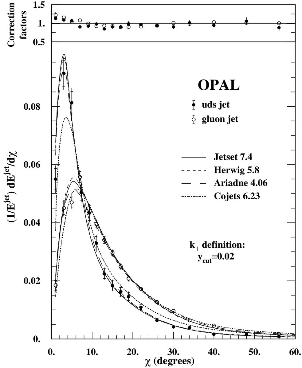
Figure 13: The normalized distribution of jet energy with respect to the jet axis for uds and gluon jets defined using the  $k_{\perp}$  jet finder; The errors shown include both the statistical and systematic terms; the experimental statistical uncertainties are indicated by the small horizontal bars.
