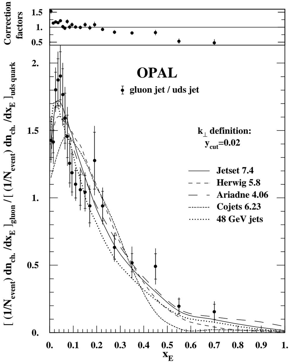
Figure 19: The ratio of the distributions shown in Fig. 18. The errors shown include both the statistical and systematic terms; the experimental statistical uncertainties are indicated by the small horizontal bars. The Jetset 7.4 prediction for 48 GeV jets, obtained by employing an  $e^+e^-$  center-of-mass energy of 180 GeV and the same event selection as applied to the other models, is also shown.
