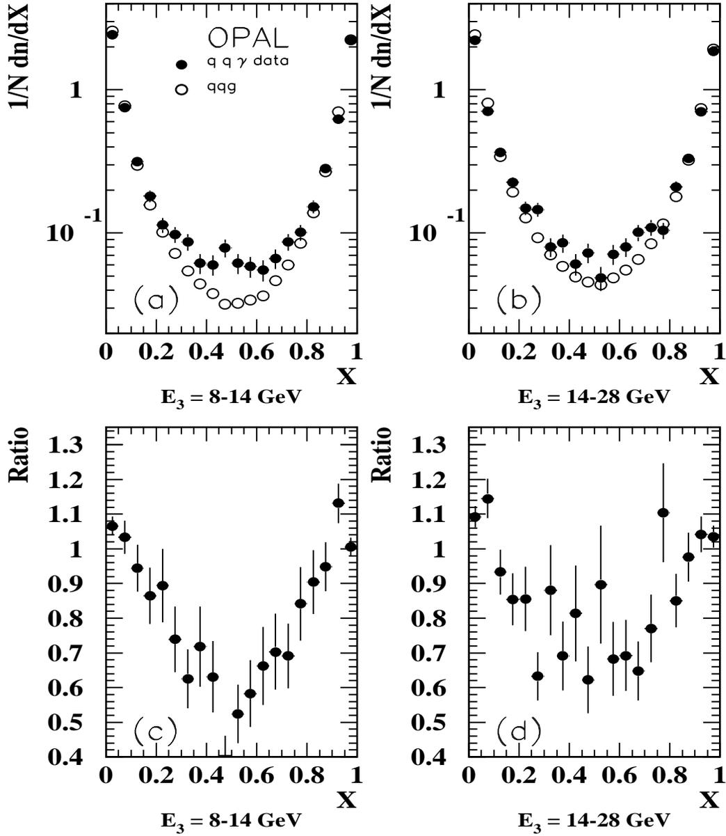
Figure 5: Charged particle flow in two ranges of  $\gamma(g)$  energies, with respect to the reduced angle  $X$  defined in the text. The bottom figures show the ratio of the two particle flows, illustrating the extent of the depletion in the  $q\bar{q}g$  sample of data.
