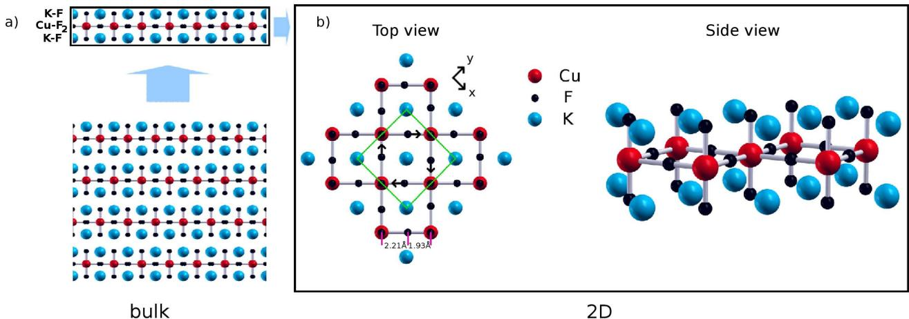
FIG. 1. (a) Crystal structure of bulk  $\text{K}_2\text{CuF}_4$  from a side view. (b) Crystal structure of 2D  $\text{K}_2\text{CuF}_4$  from the top view and side view. The green lines mark the unit cell, and the distances between the purple lines show different Cu-F bond lengths due to Jahn-Teller distortions (black arrows), which do not differ by more than 1 pm in the bulk and the monolayer. For clarity, only Cu-F bonds are visualized by gray lines.
