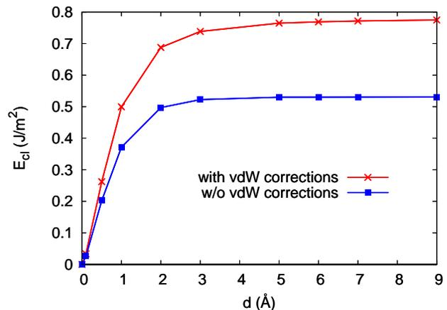
FIG. 2. Cleavage energy  $E_{cl}(d)$  as a function of the separation  $d$  of the two crystal halves.  $d$  is defined with respect to the layer-layer separation of 2.6 Å in the equilibrium configuration.
