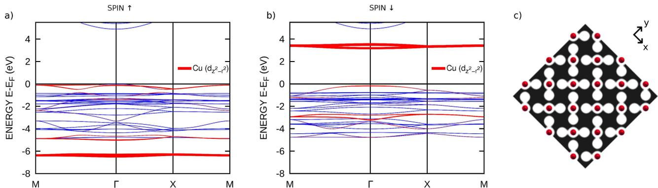
FIG. S2. a), b) Band structure of single layer  $\text{K}_2\text{CuF}_4$  in the spin up (a) and spin down (b) channel. Red "fat bands" depict the  $d_{z^2-r^2}$  contribution to the bands, whereby the thickness is proportional to the magnitude of the contribution. c) Contour plot of the hole density in the Cu-F<sub>2</sub> plane of the hole state at  $\sim 3.5$  eV shown in b) in a window between 0.35–0.55e/unit cell. Red dots denote Cu atoms.
