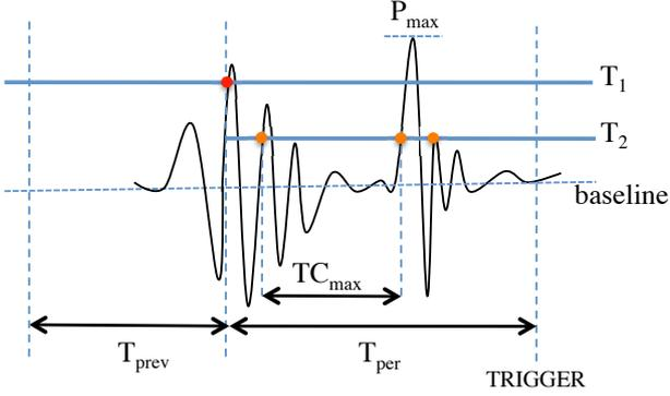
Figure 4: The AERA L1 trigger scheme. See the text for details.
