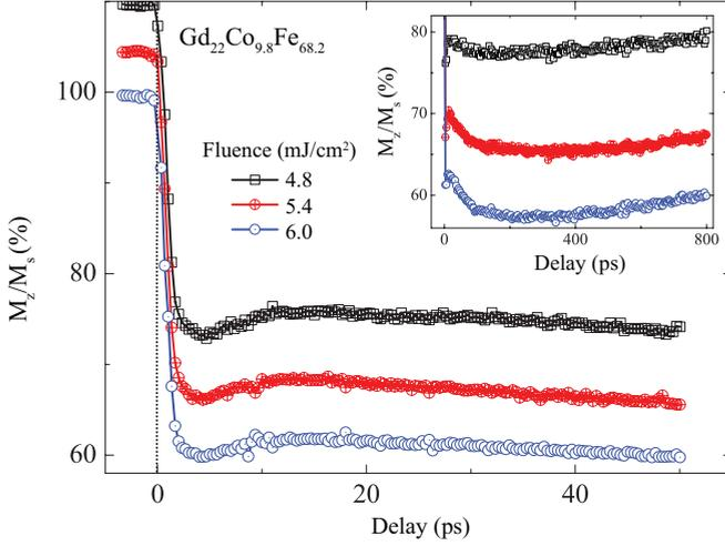
FIG. 2. (Color online) Laser-induced demagnetization as a function of pump-laser fluence in  $\text{Gd}_{22}\text{Co}_{9.8}\text{Fe}_{68.2}$ . The main panel shows the dynamics for short times, while the inset shows the one for longer times.
