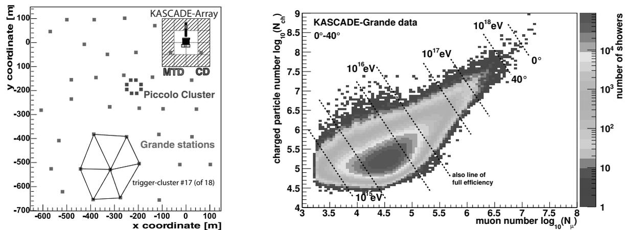
**Figure 1.** Left: Layout of the KASCADE-Grande experiment: The original KASCADE (with Array, Muon Tracking Detector and Central Detector), the distribution of the 37 stations of the Grande array, and the small Piccolo cluster for fast trigger purposes are shown. The outer 12 clusters of the KASCADE array consist of  $\mu$ - and  $e/\gamma$ -detectors, the inner 4 clusters of  $e/\gamma$ -detectors, only.
