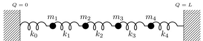
Figure 2: Mass-spring system for  $D = 4$ .
