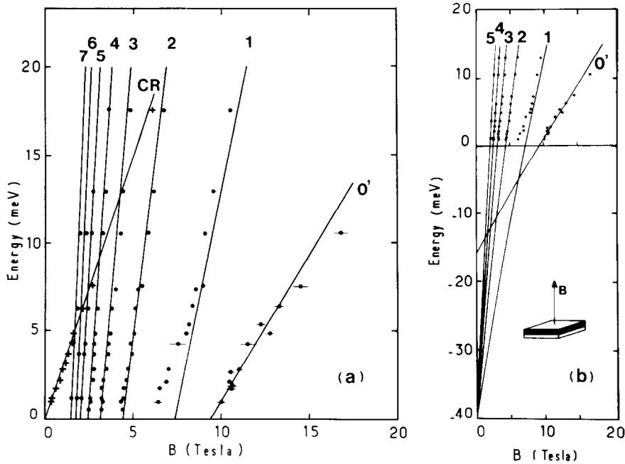
Fig. 3. Position of the transmission minima (see Fig. 2) as a function of the infrared photon energy and magnetic field  $B$  (crosses and full dots). The solid lines correspond to theoretical fits using the model presented in the text. The inset shows schematically the geometry of the experiment.
