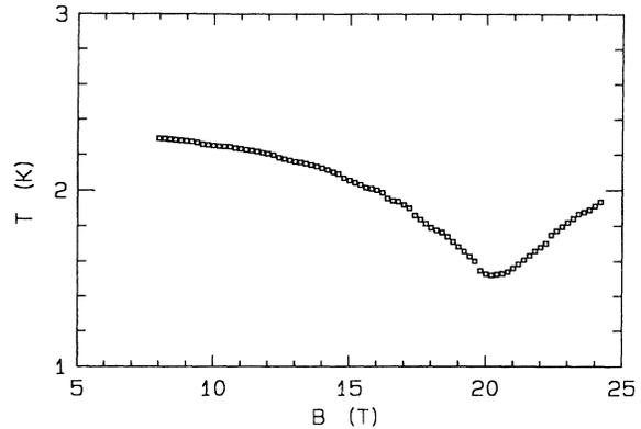
FIG. 2. The magneto-caloric effect of an adiabatically mounted single-crystalline  $\text{UPt}_3$  sample with the field  $B$  applied parallel to the  $a$  axis; the shift in temperature as a function of the applied field can be evaluated by the thermodynamic relation:  $\Delta T = -(TB/c)\partial M/\partial T$ , with  $M$  the sample magnetization and  $c$  the specific heat.
