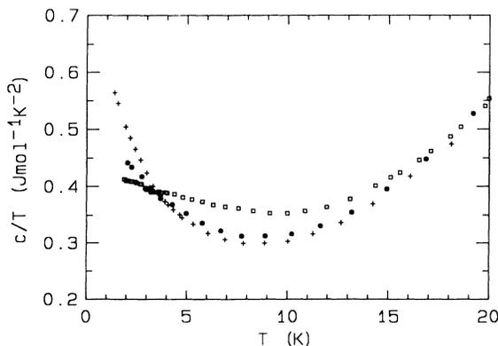
FIG. 1. The specific heat of single-crystal  $\text{UPt}_3$  in a plot of  $c/T$  vs  $T$  at different field strengths:  $\square$  (0 T);  $+$  (20 T);  $\bullet$  (24.5 T); fields have been applied along the  $a$  axis in the hexagonal plane.
