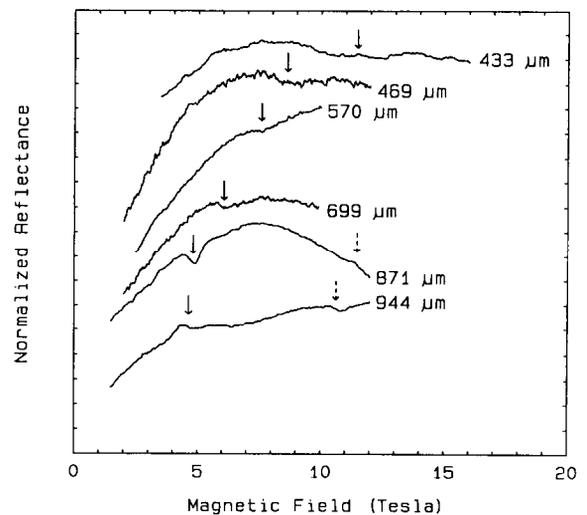
Fig. 2. Normalized magneto-reflectance of  $ET_2KHg(SCN)_4$  at 1.2 K for different radiation energies. The primary series of CR features are marked with solid arrows and additional features with broken arrows.
