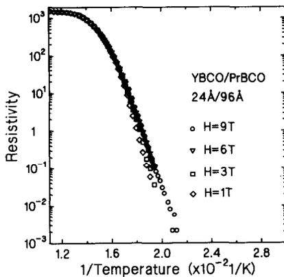
Fig. 7. Resistivity  $\rho(T, H)$  versus  $1/T$  for a 24 Å/96 Å superlattice for different magnetic fields applied parallel to the  $a, b$  plane (0, 1, 3, 6 and 9 T).
