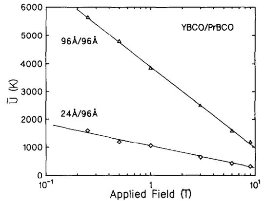
Fig. 6. Activation energy versus  $\log B$  for a  $24 \text{ \AA}/96 \text{ \AA}$  and a  $96 \text{ \AA}/96 \text{ \AA}$  superlattice. The magnetic field is applied perpendicular to the  $a, b$  plane.
