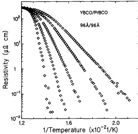
Fig. 4. Resistivity  $\rho(T, H)$  versus  $1/T$  for a  $96 \text{ \AA}/96 \text{ \AA}$  superlattice and for fields of 0, 1, 3, 6, and 9 T. The magnetic field is applied parallel to the  $c$ -axis.
