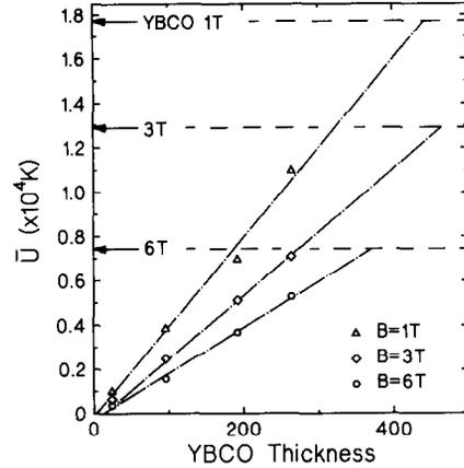
Fig. 5. Activation energy at 1, 3 and 6 T as a function of the YBCO thickness in multilayers with thick PrBCO separation thicknesses. The arrows show the values for a  $1500 \text{ \AA}$  YBCO thick film. The magnetic field is applied perpendicular to the  $a, b$  plane.
