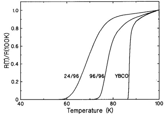
Fig. 1. Resistive transitions for a 24 Å/96 Å and a 96 Å/96 Å superlattice compared to the transition of a YBCO film.
