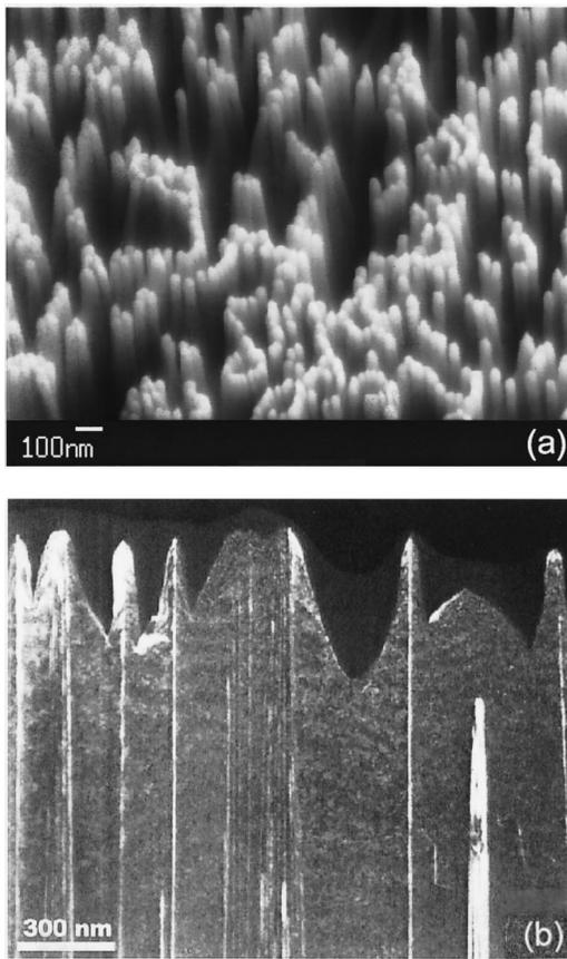
FIG. 1. (a) SEM image of dislocation-related PEC etched whiskers on the Ga-polar GaN heteroepitaxial layer. (b) Weak beam cross-sectional TEM image ( $\sim g/4g$ , with  $g = [11-20]$ ) of PEC etched Ga-polar layer: one-to-one correlation of dislocations to whiskers. Some dislocations end before reaching the top of whisker, indicating a foil cutoff by ion milling.
