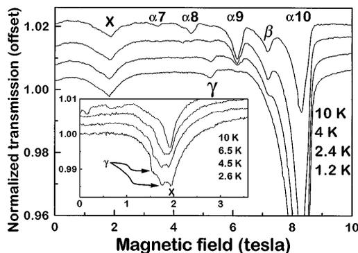
FIG. 4. Magnifications of intermediate frequency EPR data obtained for each orientation; for  $\mathbf{B}_0 \perp \mathbf{c}$  (main part of figure), the frequency is 57.4 GHz; and for  $\mathbf{B}_0 \parallel \mathbf{c}$  (inset), the frequency is 55.16 GHz. The temperatures are indicated in the figures. Also, see text for explanation of labeling.
