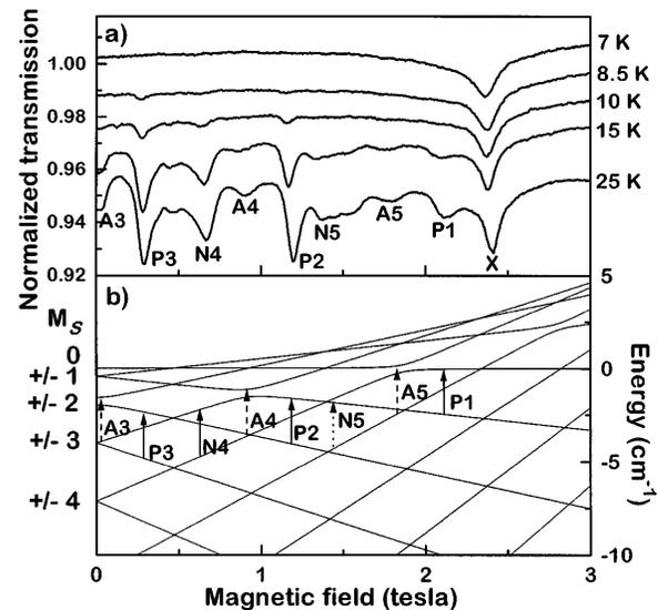
FIG. 1. (a) Temperature dependence of the normalized transmission (offset) for  $\mathbf{B}_0 \parallel c$ ; the frequency is 66.135 GHz. (b) A calculation of the corresponding energy levels for the  $S = 10$  spin system [13]; the arrows indicate transitions responsible for the resonances in (a). See text for details of the calculation and for an explanation of the labels.
