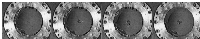
FIG. 4. Macroscopic nucleus formation from beads (5 mm). The conditions are similar to those in Fig. 3. The object at magnet center is a U.S. dollar bill, which is paramagnetic and is attracted to the bore tube wall.
