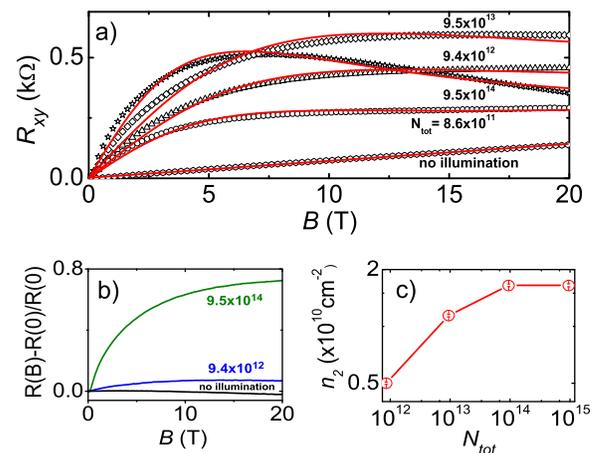
FIG. 3. (a) Hall resistance data as a function of the applied magnetic field, for illumination with different values of  $N_{tot}$  with energy of 3.65 eV at 4.2 K (open symbols). Solid lines: The two-band model fits to the experimental data. (b) (longitudinal) Magnetoresistance data as a function of the applied magnetic field and (c) carrier concentration of the second, high mobility band for illumination with different values of  $N_{tot}$ .
