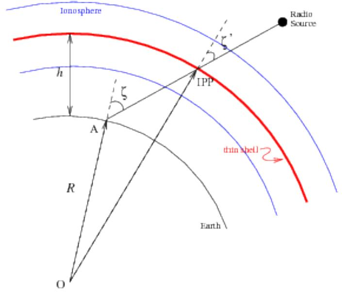
**Fig. 1.** Schematic representation of an astronomical signal piercing the ionosphere. The solid blue curves delineate the ionosphere. The thick red curve is the ionospheric thin shell approximation, and the thin black curve delineates the surface of the Earth.
