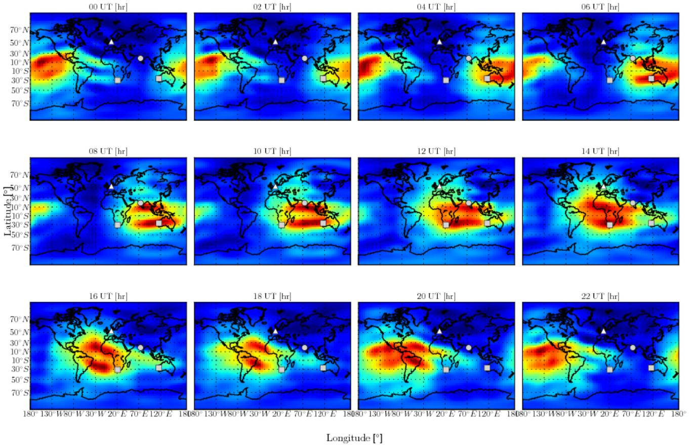
**Fig. 2.** GIMs representing the VTEC across the globe for April 11th, 2011 (the date of the first LOFAR observing campaign, see §5) obtained courtesy of CODE. The maps range from minimum (blue) to maximum (red) VTEC values of 0.0 – 87.2 TECU (1 TECU =  $10^{16}$  electrons/m<sup>2</sup>). The triangles indicate the location of the LOFAR core stations in the Netherlands, the squares mark the SKA core sites in South Africa and Western Australia, and the circles indicate the site of the GMRT.
