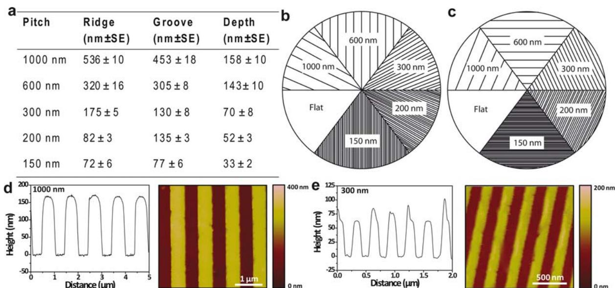
**Fig. 1.** **a.** Groove dimensions  $\pm$  standard error of the mean. **b, c.** Schematic diagram of multi-patterned substrates. **d, e.** Cross-sections and height images of the nanopatterns created by AFM imaging.
