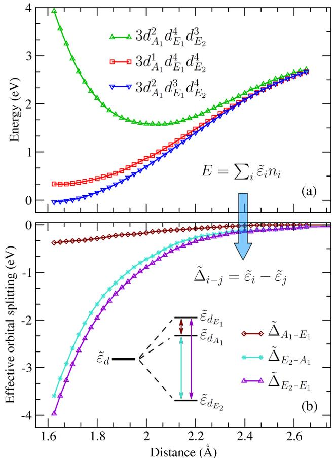
FIG. 5. (Color online) (a) Potential energy curves for different orbital occupations of Co in the  $3d^9$  configuration; (b) energy differences between nonequivalent  $3d$ -orbital levels of Co (the effective crystal-field splitting parameters) calculated as functions of the adatom–surface separation (see text for details). The splitting of the energy levels is shown schematically inside the lower panel.
