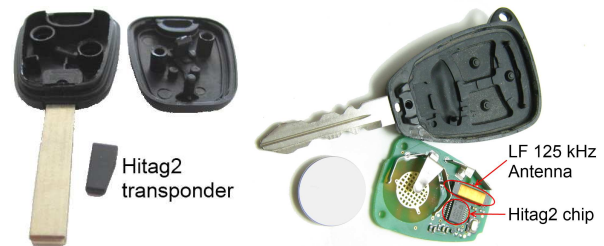
Figure 1: Car keys with a Hitag2 transponder/chip
