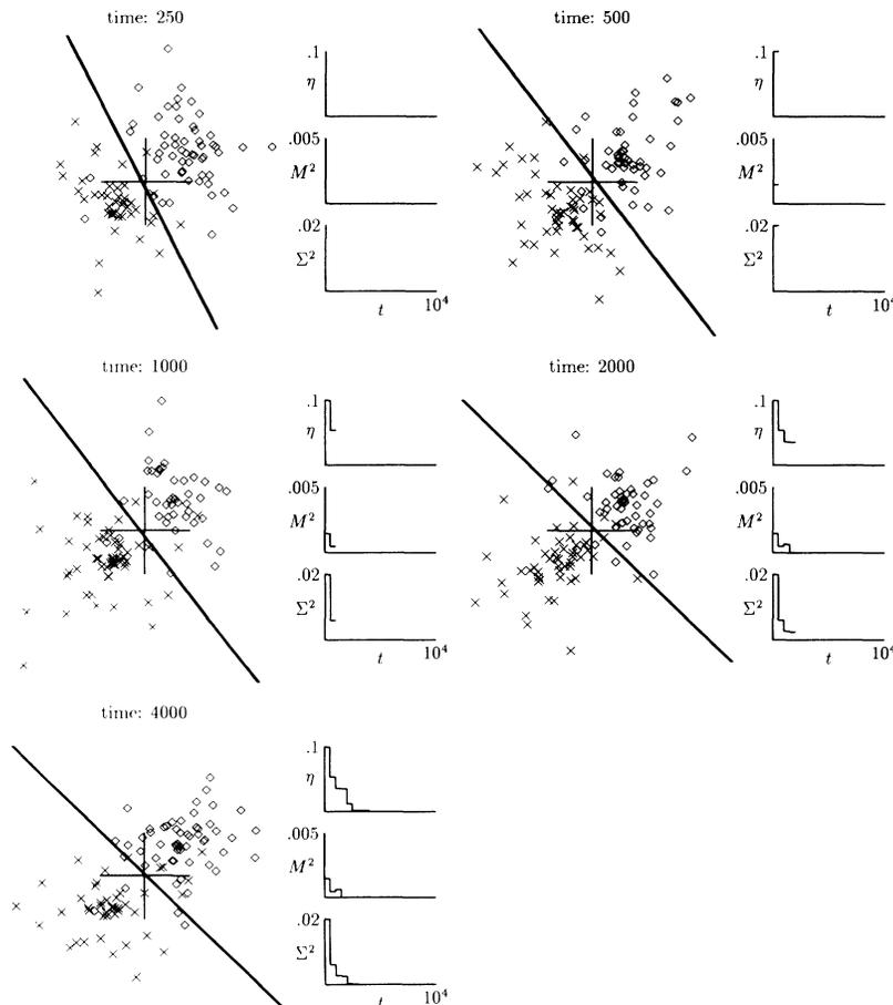
FIG. 1. A fixed environment:  $\phi(t) = \phi(0) = \pi/4$ . The bold line is the decision boundary found by the network. The last 100 training patterns are shown; diamonds represent positive outputs, crosses represent negative outputs. Graphs on the right give the learning parameter, squared bias, and variance as a function of time, all calculated from the statistics of the weights. Variance of input examples  $\sigma=1$  and time window  $T=500$ .
