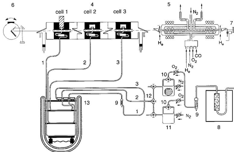
Fig. 1. Detection setup: 1, 2, and 3, trace-gas flows; 4, triple photoacoustic cell; 5, liquid-nitrogen-cooled CO laser; 6, grating to select the appropriate transition; 7, chopper; 8, catalyst to remove hydrocarbons; 9, KOH scrubber to remove  $\text{CO}_2$ ; 10, switching valve for (an)aerobic conditions; 11, cuvettes, one containing a tomato, the other empty as a reference; 12, switching valve to select the cuvette; 13, cooling trap.
