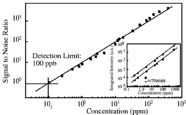
Fig. 3. Signal-to-noise ratio of  $\text{NH}_3$  peak absorption for averaged fast scans (5 nm/min). The inset shows integrated intensity versus concentration (units differ for HITRAN96 simulations and PAS owing to nonabsolute concentration calibration).
