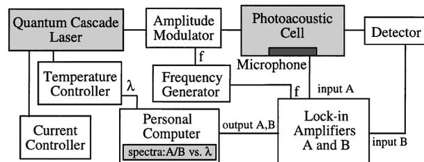
Fig. 1. Block diagram of the photoacoustic apparatus.
