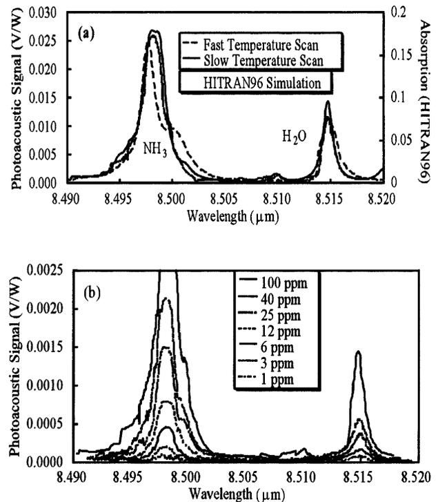
Fig. 2. Photoacoustic spectra of NH<sub>3</sub> and H<sub>2</sub>O diluted with nitrogen at STP: (a) slow (0.5-nm/min) and fast (5-nm/min) temperature tuning spectra compared with HITRAN96 simulations (50-ppm ammonia mixture), (b) slow-scan spectra corresponding to various mixture dilutions. All lines are pressure broadened to several gigahertz.
