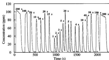
Fig. 4. Real-time  $\text{NH}_3$  concentration monitoring by use of the  $8.498\text{-}\mu\text{m}$  peak absorbance for a 100-ppm  $\text{NH}_3\text{-N}_2$  mixture injected into a  $\text{N}_2$  stream. The mixture bolus injection time is indicated for each cycle. The cell was operated at STP (2-L/h flow rate). The gas mixture was interrupted with a mechanical valve.
