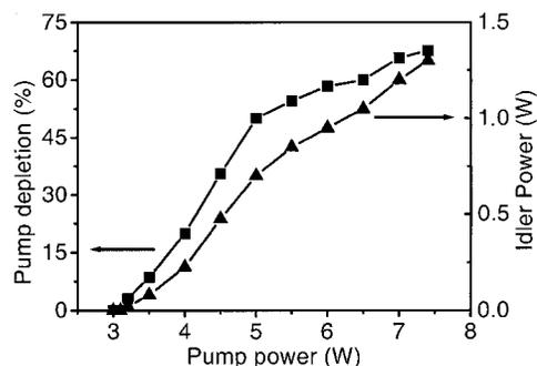
Fig. 2. Idler output and pump depletion versus pump input power for the SRO operating at an idler wavelength of 3.3  $\mu\text{m}$ . The oscillation threshold is 3.0 W, and a maximum idler power of 1.5 W is observed with a pump power of 9 W.
