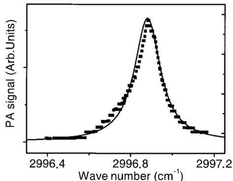
Fig. 3. Single-frequency tuning of the pressure-broadened (0.75-atm)  $\nu_7$ ,  $v = 1 \leftarrow 0$ ,  $K = 4 \leftarrow 3$ ,  $Q$ -branch transition ( $J = 4-39$ ) of ethane is demonstrated by use of photoacoustic (PA) spectroscopy. The experimental results are shown by the scatter graph, and the spectrum of ethane from the Hitran database is shown by the solid curve.
