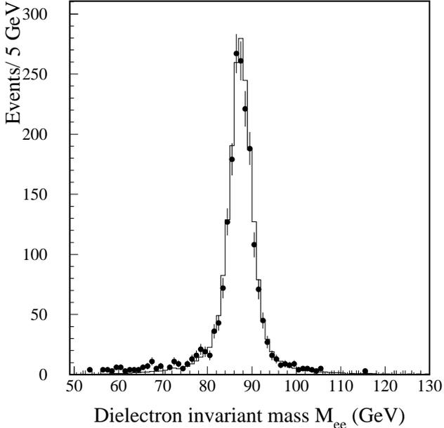
FIG. 3. Invariant mass distribution of  $Z \rightarrow e^+e^-$  events compared to Monte Carlo simulation. The histogram is the MC and the black dot with error bar is the data. The  $Z \rightarrow e^+e^-$  candidate require both electrons be in the CC.
