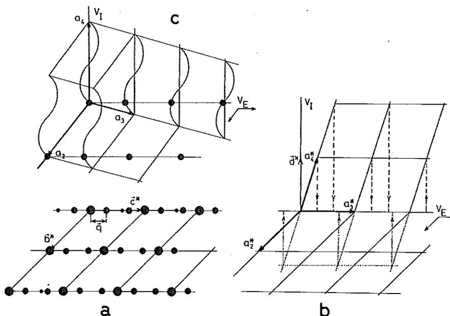
FIGURE 1 a) X-ray diffraction pattern of incommensurate crystal with  $\vec{q} = \gamma\vec{c}^*$ . Big dots indicate main spots, smaller dots indicate satellite reflections. b) Construction of superspace reciprocal lattice corresponding to diffraction pattern of 1a. c) Superspace crystal; dots indicate the real atom positions, obtained by intersecting the wavy pattern of the s.s. crystal with  $V_E$  (here and in 1b  $V_E$  is drawn as a 2-dimensional plane).
