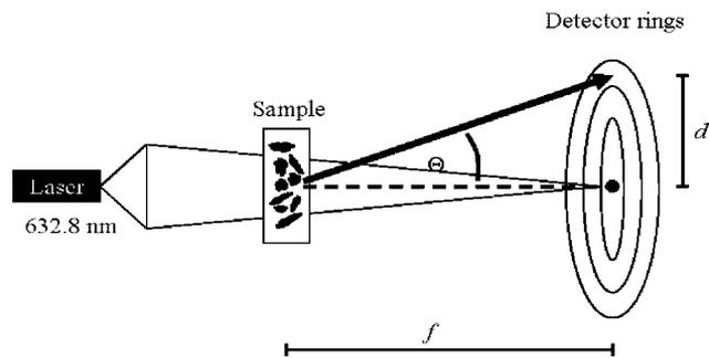
Fig. 1. Optical setup of the laser particle sizer.
